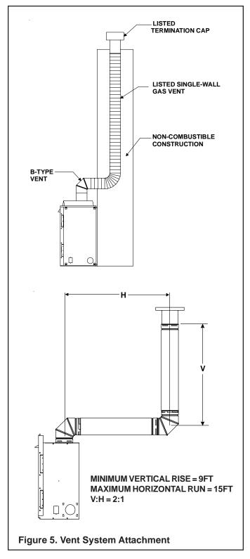
NOTE: The vent termination must be in a vertical position and the termination cap must be listed for the vent pipe used.
